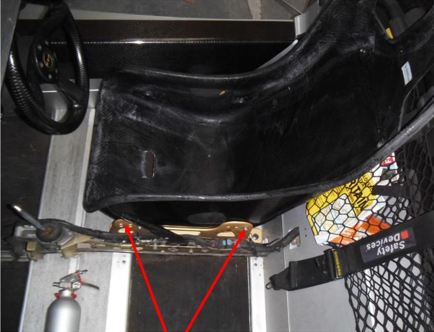
once the subframe bolted tight to the floor pan then the subframe can be tightened to the seat.
